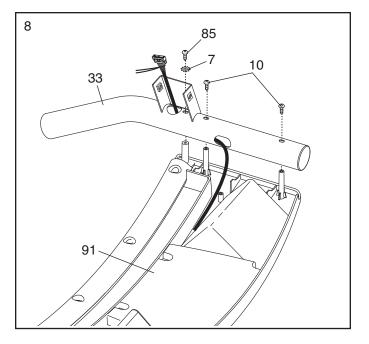
Remove the ties from the Cage Nuts (103) in the Right Handrail (33) and the Left Handrail (not shown). If necessary, press the Cage Nuts back into place. With the help of a second person, hold the Console Assembly (91) near the Right Upright (54).
